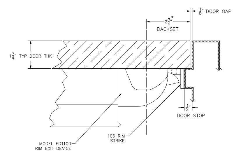
BACKSET IS BASED ON THE LISTED DIMENSIONS FOR DOOR STOP & DOOR GAP. NEED TO COMPENSATE FOR VARIATIONS IN THOSE DIMENSIONS.
