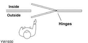
If hinges are on the left, and the door opens inward or outward it is a **left** hand door (LH)
