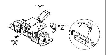
Remove the "X" screw, pull out "Z".
