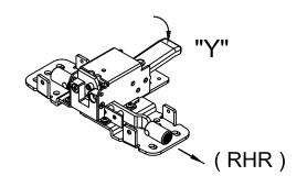
Press Lift Arm "Y" to ensure handing is correct.
