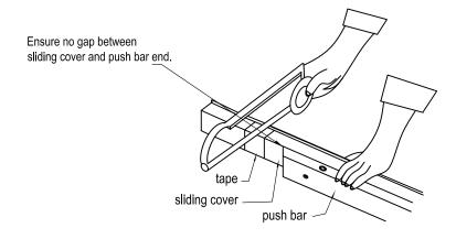
NOTE: the minimum length of the sliding cover must be 1"(25.4mm) or longer than length "C".
