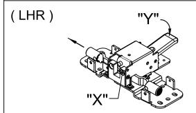
Press Lift Arm "Y" and ensure the direction before changing. The "X" screw is located shown for LHR.
