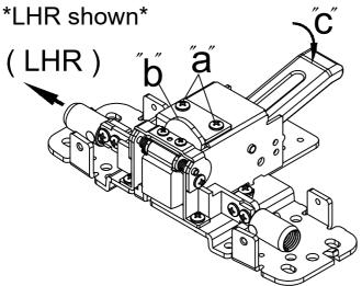
Press Lift Arm "c" and ensure the direction before changing.
