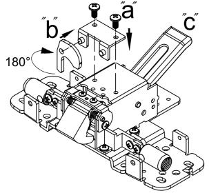
Turn "b" 180° and put it back as figure shown. Fasten "a" at above screw hole position.
