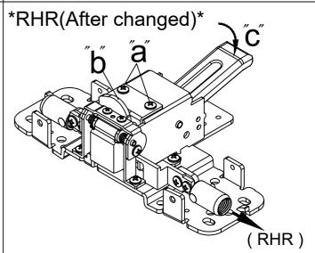
Press Lift Arm "c" to ensure the processing direction is reversed.
