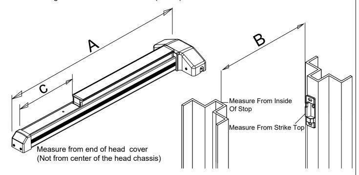
2.2 If required cut C length of device so A is at least 1- 3/4" (45mm) shorter than B.
