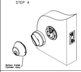
Place inside t-turn or optional inside cylinder assembly over mounting plate.
