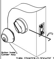
There are 2 holes on each side of the t-turn assembly (or optional inside cylinder assembly). Use the provided 5/64" allen wrench- stick it into the hole and engage the set screw on the mounting plate. Thurn the set screw counter-clockwise to secure the the t-turn. Do this on both sides. Do not over tighten. Turn the set screws clockwise to un-install.
