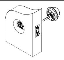
Install outside cylinder assembly as shown. Spindle blade is in the vertical position and goes through the driver on the deadbolt.
