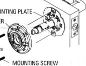
b. Use lever catch to press down catch in the hole and push inside lever all the way in until clicks into catch hole.
