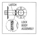
Repeat No. 6 to intall the removable Thru-Bolt. Install outside lever assembly on the door. Make sure tail of latch engaging with retractor correctly as illustration **OUTSIDE** left. LEVER
